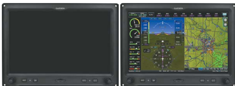
G3X Touch Full-Screen Reversionary Mode (Failed PFD)
