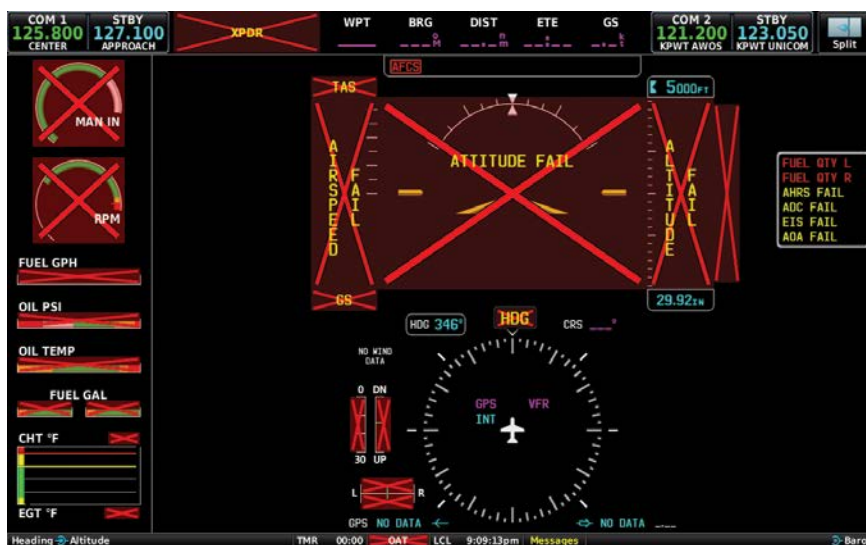
G3X Touch System Failure Annunciations
