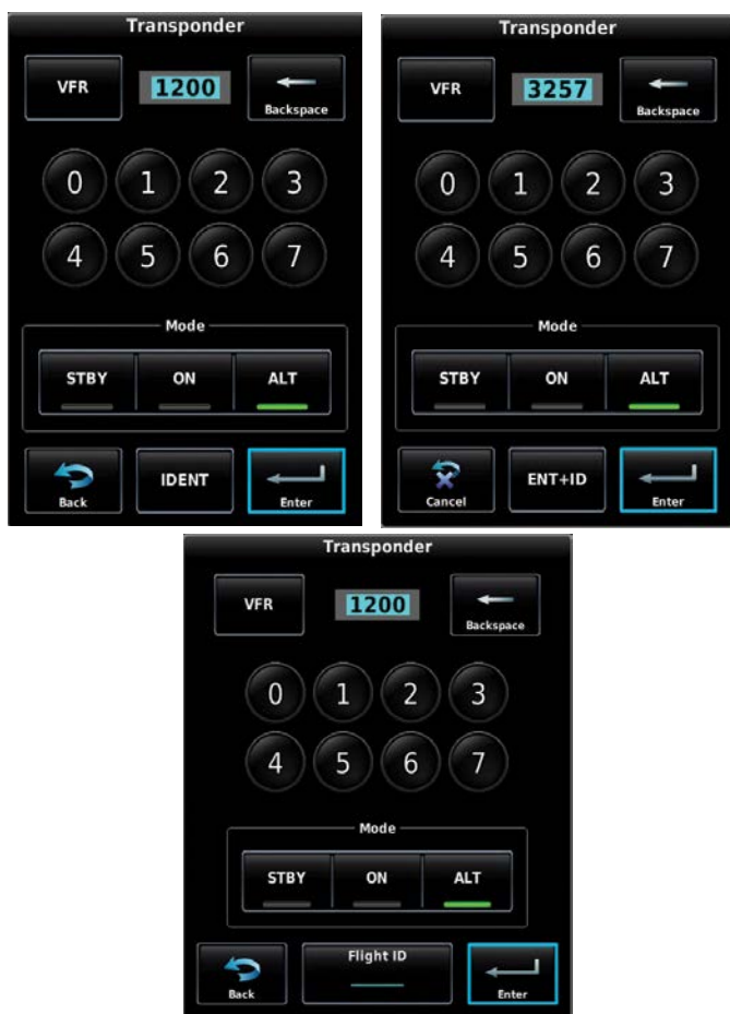
Transponder Code, Mode, and Flight ID Entry
