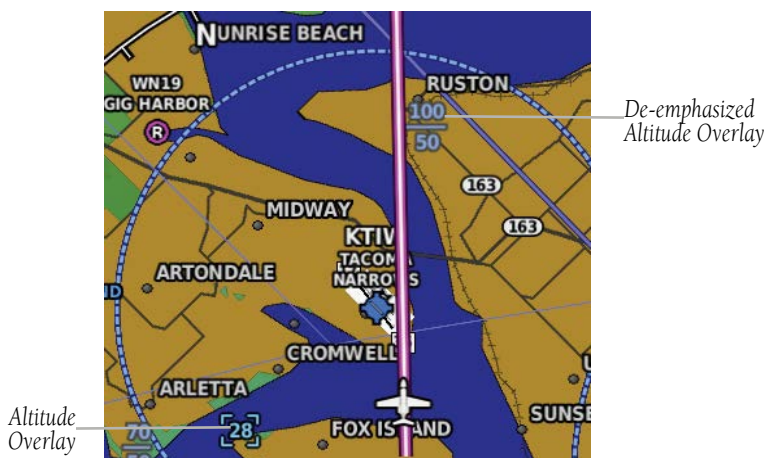
Smart Airspace™ with Altitude Overlays
