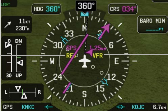
External GPS Navigator Failure
