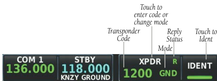
Transponder Data Box on CNS Bar
